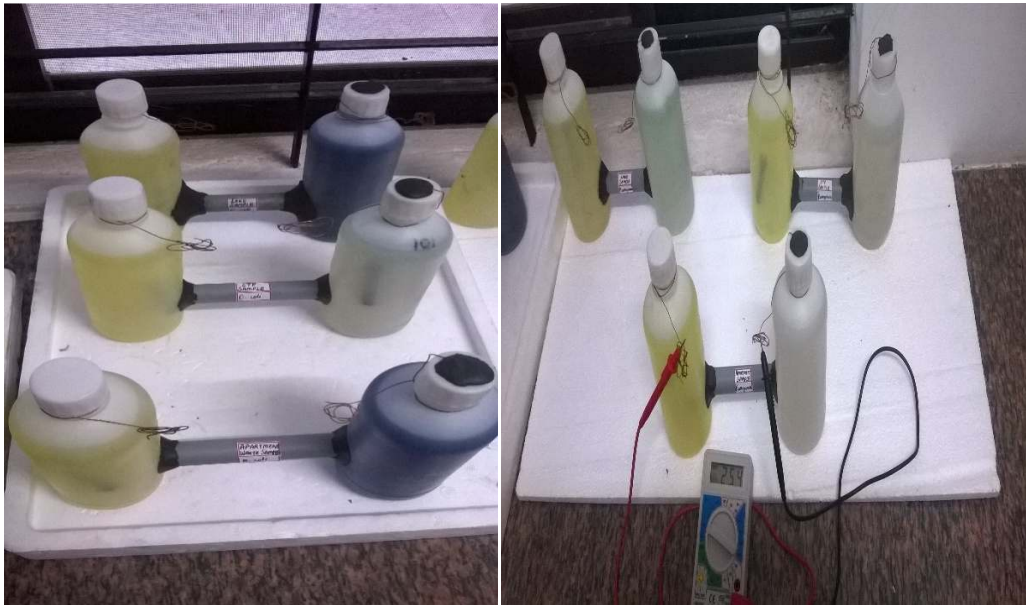
Fig. 2. Construction of double chamber setup
