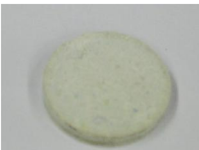
Fig. 2. Shows the ITO target used in the pulsed laser deposition process.
