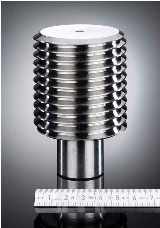
Figure 3. Screw thread gauge used for the verification of the novel 3D inspection method.
