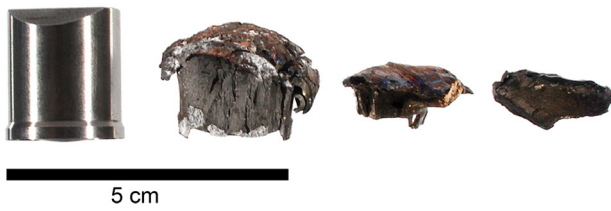
Figure 2. Exemplary image of the steel cylinder before impact (leftmost item) and the three largest fragments formed during an impact process (to the right). Reproduced with permission from [26].
