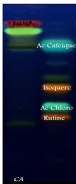
Fig. 2c. Flavonoids SP: Silicagel 60F 254 MP: Ethyl acetate / Methanol / Water / Formic acid Developer: Neu reagent
