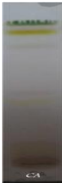
Fig. 2b. Iridoids SP: Silica gel 60F 254 MP: Acetated ethyl / Formic acid / Water Developer: Sulfuric acid
