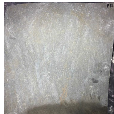
Back of Greenkote (Phosphate) Plate After Testing
