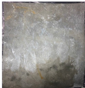
Front of Greenkote (Phosphate) Plate After Testing
