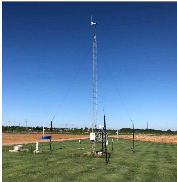
Figure 2. Automatic weather station (AWS) used to measure hourly values of weather variables and compared to measurements obtained with four PWS located at the Cropping Systems Research Laboratory, Lubbock, TX (Photo courtesy of Dr. John E. Stout).
