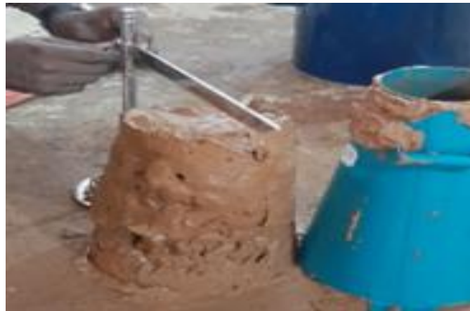
Fig. 1. Slump of fresh geopolymer concrete mix
