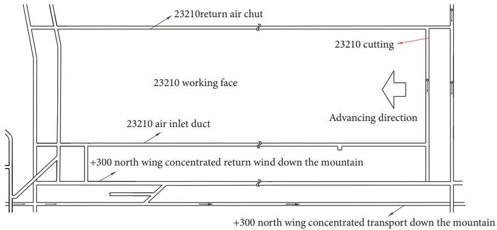
FIGURE 2: Schematic diagram of 23210 working face.
