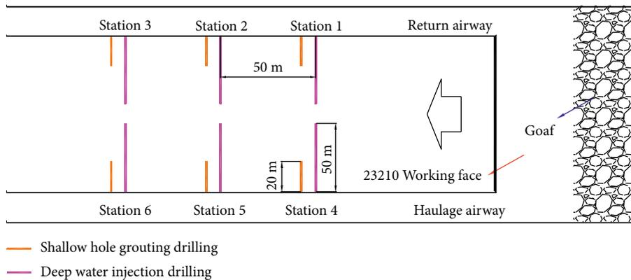
FIGURE 10: Schematic diagram of prevention and control measures of working face.
