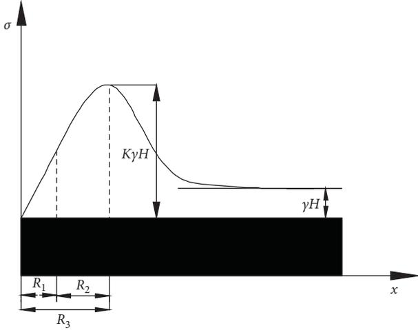
FIGURE 4: Coal body division and abutment pressure distribution.
