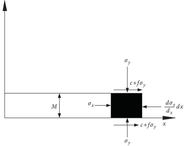
FIGURE 5: Force analysis of coal unit.
