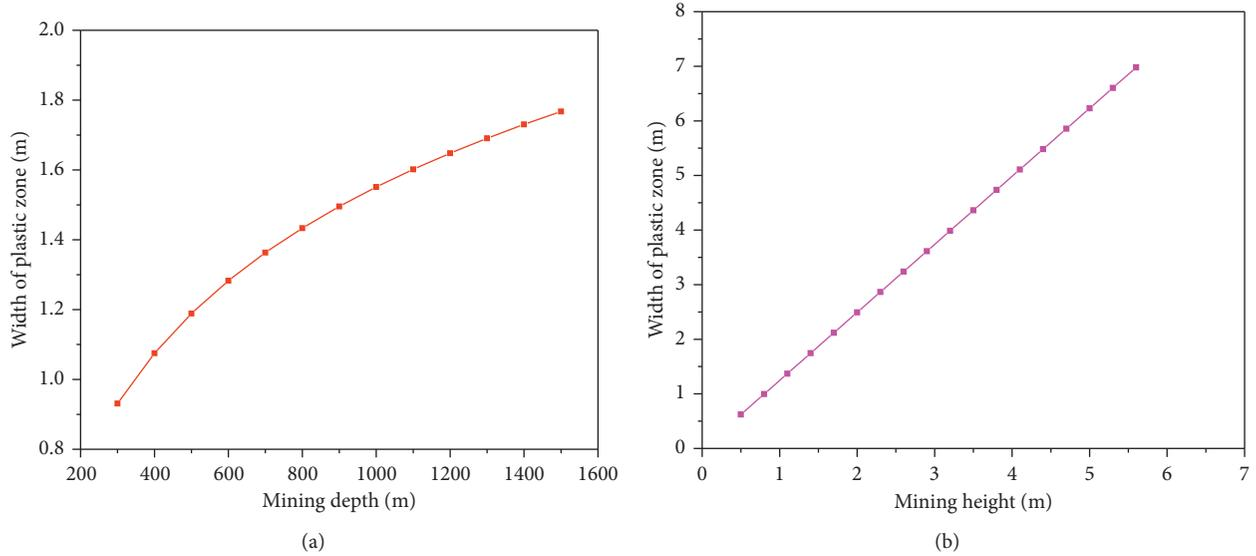
FIGURE 6: Relationship between width of plastic zone and mining depth and mining height.
