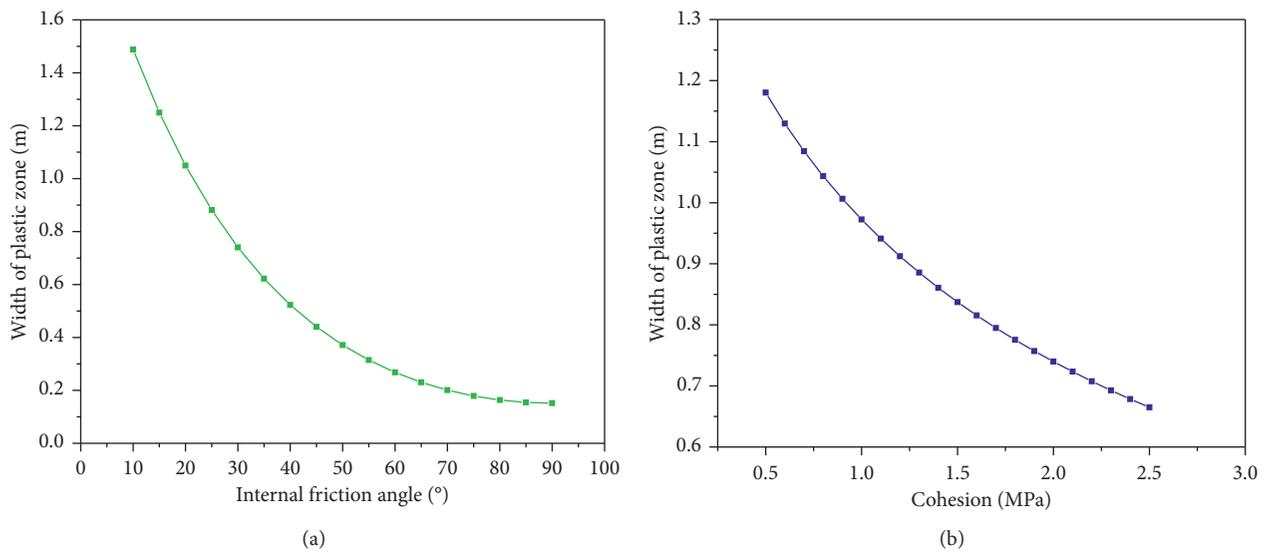
FIGURE 7: Relationship between width of plastic zone and internal friction angle and cohesion.
