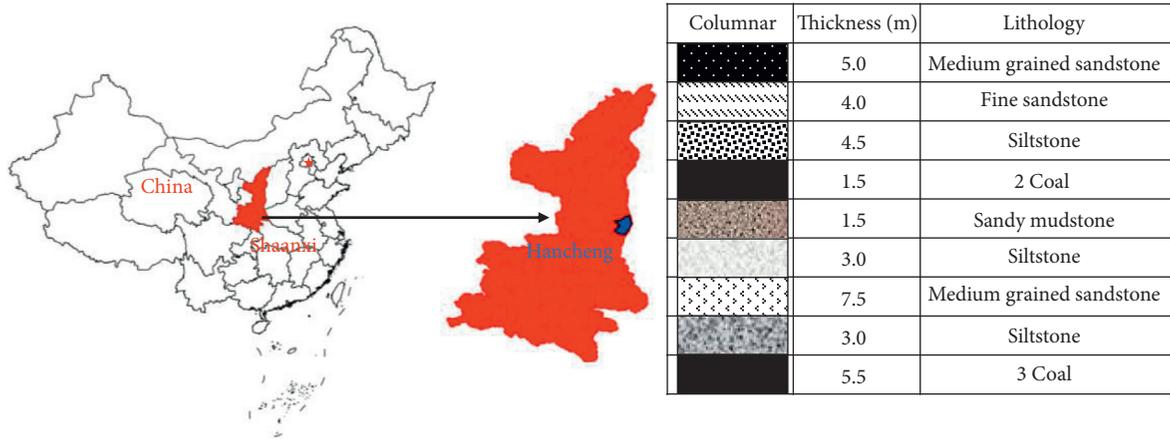
FIGURE 1: Location of the coal mine and its general stratigraphic column.
