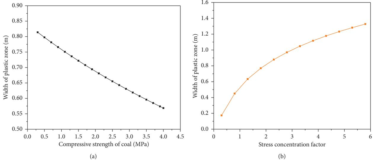
FIGURE 8: Relationship between width of plastic zone and compressive strength and stress concentration factor.
