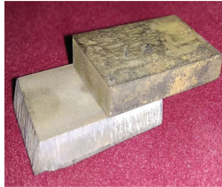
FIGURE 4: Lap shear tensile test specimen details.
