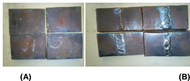
Fig. 1a(A-B). Sample of mild steel plate of IS2062 E-250 and its welding samples
