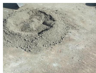
(c) Mixture of cement, recycled glass powder and fine aggregates
