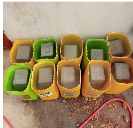
(b) Curing of specimens
