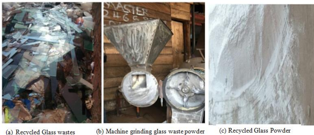
Fig. 2. Recycled glass powder used for the study
