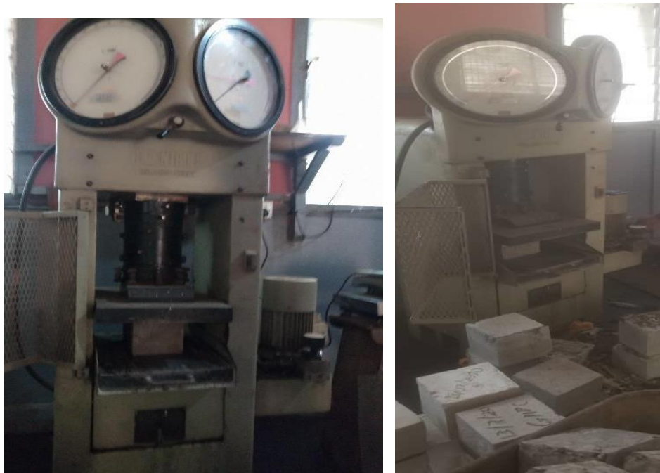
Fig. 7. Concrete cube specimens under test
