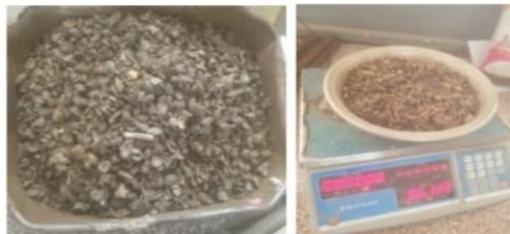
Fig. 3. Selected Palm Kernel Shells being weighed
