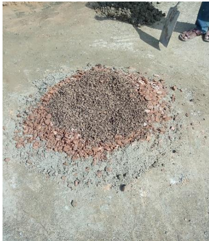
(d) Coarse aggregate and Palm kernel shells added to the mixture of cement, recycled glass palm powder, and fine aggregate
