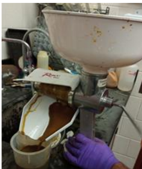
Fig. 5. Hand operated screw press [21]
