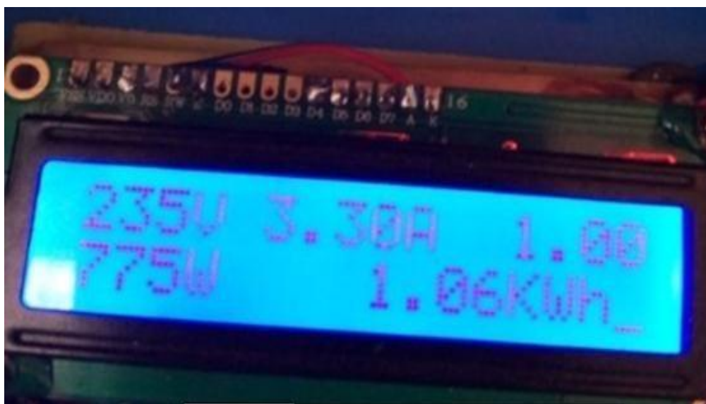
Fig. 7. Snap shot of prototype meter lcd display of voltage, current, pf, 'real-time' power and electrical energy
