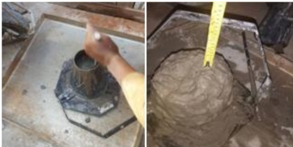
Fig. 5. Slump test being conducted on fresh concrete
