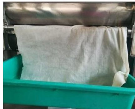
Fig. 1 b) Bamboo fabric passed through pneumatic padding mangle
