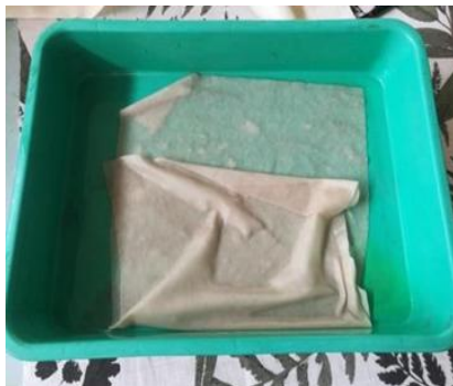
Fig. 1 a) Bamboo fabric dipped in silver nanoparticle solution
