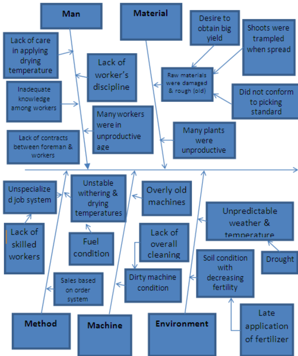
Fig. 2. Fishbone diagram of Pekoe product that was inferior to standard
