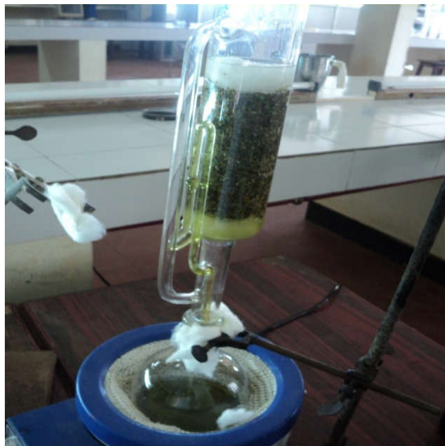
Fig. 2. Preparation of ethanolic extract of S. acmella using a Soxhlet apparatus
