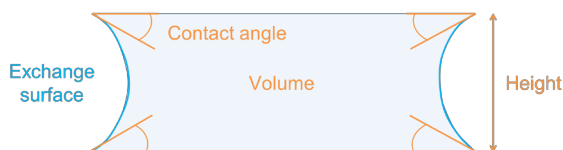
Figure 6. Liquid bridge geometric parameters which have been investigated in the present study.
