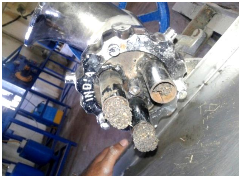
Fig. 3. Briquettes coming out from the developed briquetting machine
