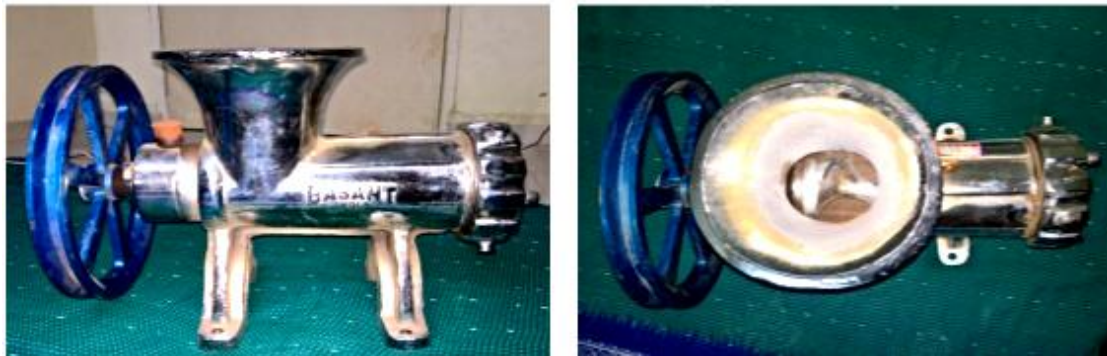
Fig. 1. Developed briquetting machine
