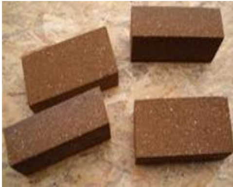
Fig. 1. Pictures of compressed soil building blocks used as samples
