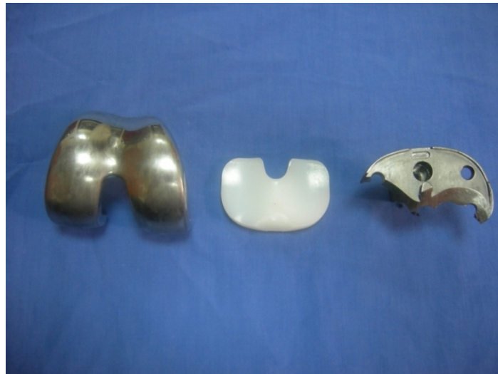
Fig. 4. The appearance of defect at the tibial component and an intact polyethylene insert
