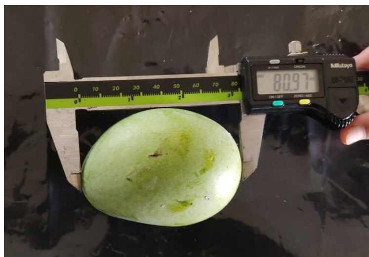
Plate 3. Measurement of fruit length by using a digital slide caliper
