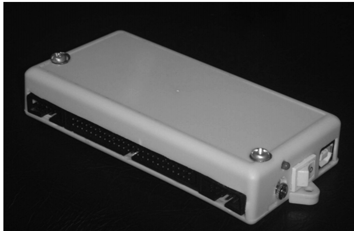
Fig. 2. Shows the device to record and transfer data to computer.
