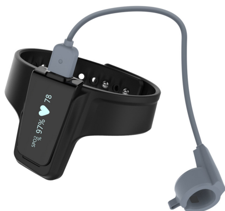
Figure 5. The Viatom Checkme O2 device to monitor blood oxygen level, heart rate, and movements.
