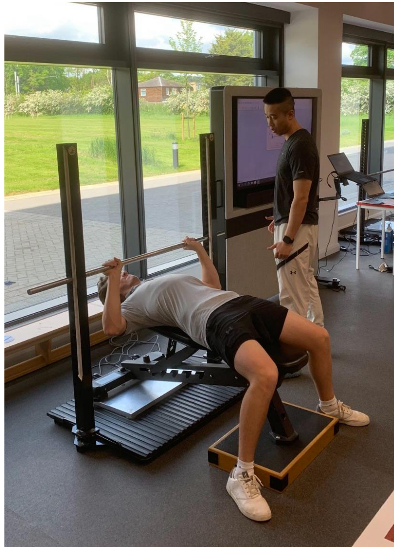
Figure 2. Set-up of the isometric bench press assessment.
