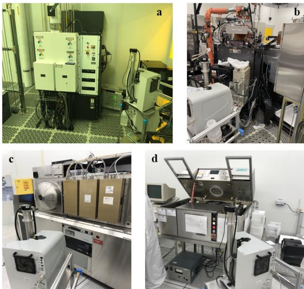
Figure 2. SMPS configuration employed for field observation at the (a) PECVD (I), (b) Fluorine etching, (c) sputtering (I), and (d) plasma etching areas in the MTW cleanroom.
