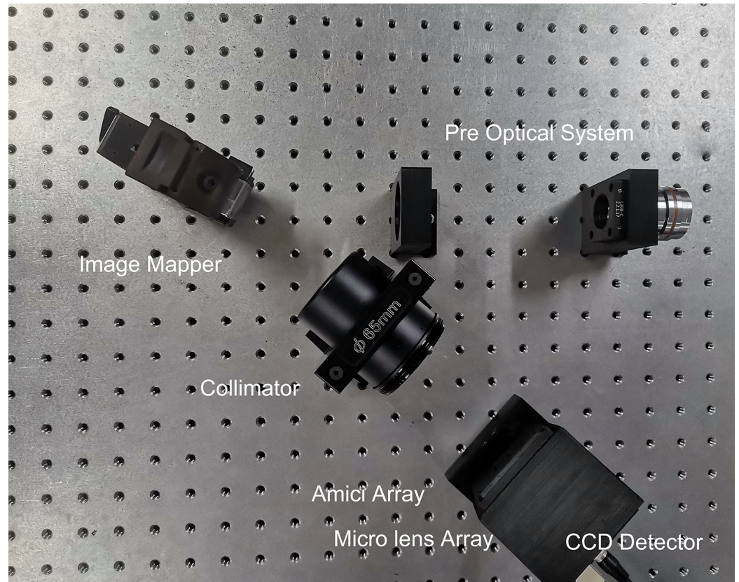
Figure 8. IMS experimental system includes Pre Optical System, Image Mapper, Collimator, Amici Array, Micro Lens Array and Image Detector.
