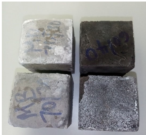
Fig. 3. Cube sample efflorescence
