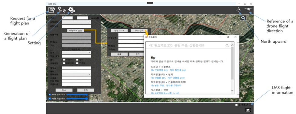
Figure 2. Graphic UI (User Interface)—GCS (Ground Control Stations).
